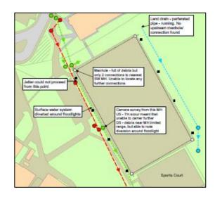
The second was traced back to a previous misconnection of foul waste from a neighbouring commercial premises to the storm water system that runs through the Sue Noake site alongside the ATP (see red dots in Diagram ---).
